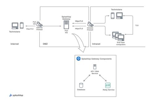
Both inbound and outbound communication between all the components is encrypted.
